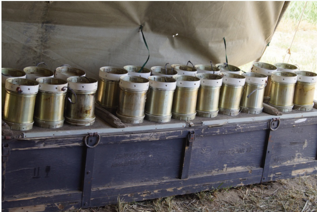
Warheads of R60/R73 missiles without depleted uranium after safe disassembly
