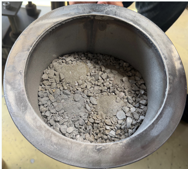
RDX (hexogen) explosive removed from 30 mm ammunition after final disposal operation
