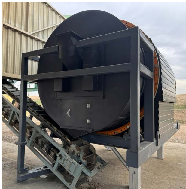
Armored furnace with a cylindrical steel armor 20 mm, to protect against fragments, installed in Arys.
