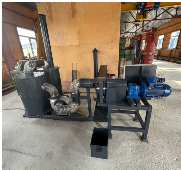
Machine for shooting capsule sleeves with aspiration system for disposal of 23-30 mm ammunition.
