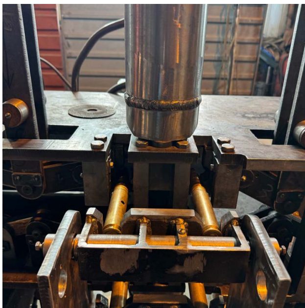
Machine for unscrewing fuses, unloading and removing gunpowder for disposal of 23-30 mm ammunition
